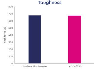
Measured using a TA.XT plus C texture analyser according to AIB bakery standards.
